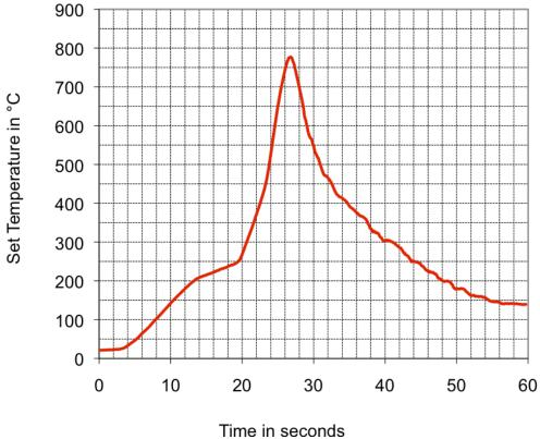
SierraTherm-5 zone IR with 25 cm peak firing zone Furnace:
